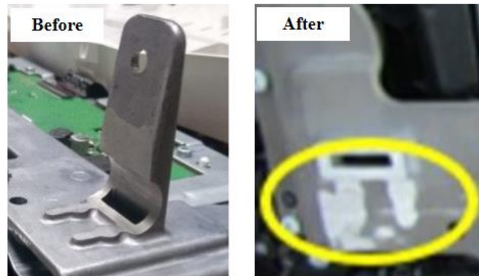
Fig. 8. Mounting Bracket Before and After impact testing
