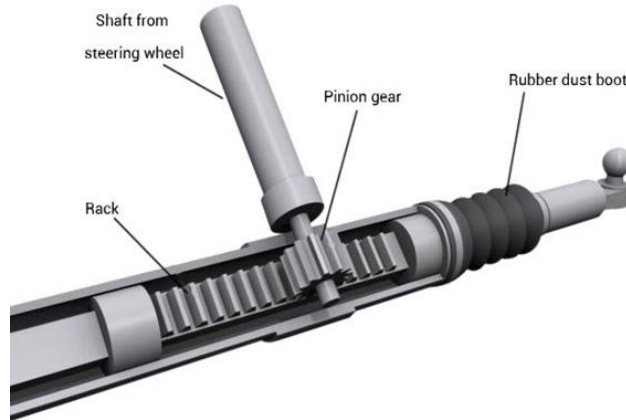
Fig 1. Working Of Rack And Pinion Mechanism
