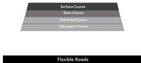
Figure 1. Typical structure of asphalt pavement [15]
