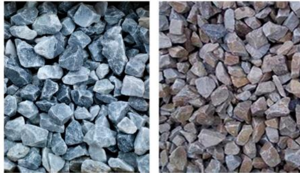
Figure 3. Quarry waste (left) and traditional aggregate (right)
