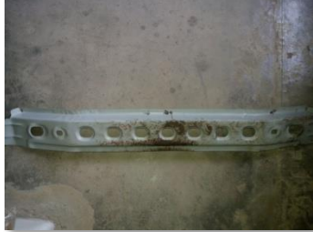
Fig.20. Original Model of the INDICA Car Bumper Beam (Model – 2015)
