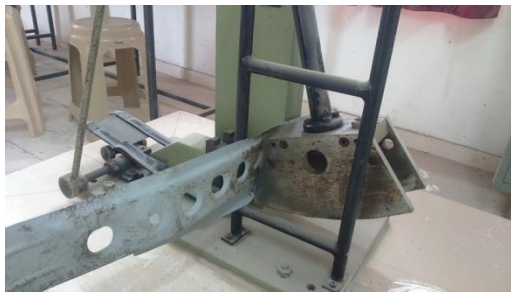
Fig.21 Bumper Beam on Impact Tester
