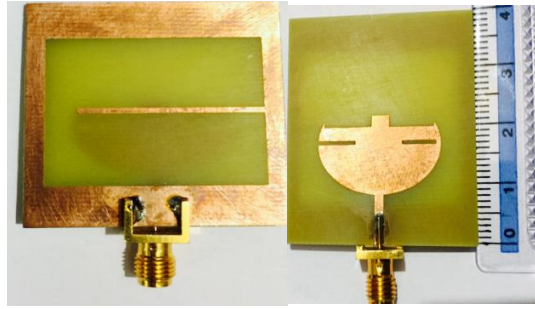
Fig.2 Photograph of Fabricated antenna (a) bottom ground layer (b) upper ground patch
