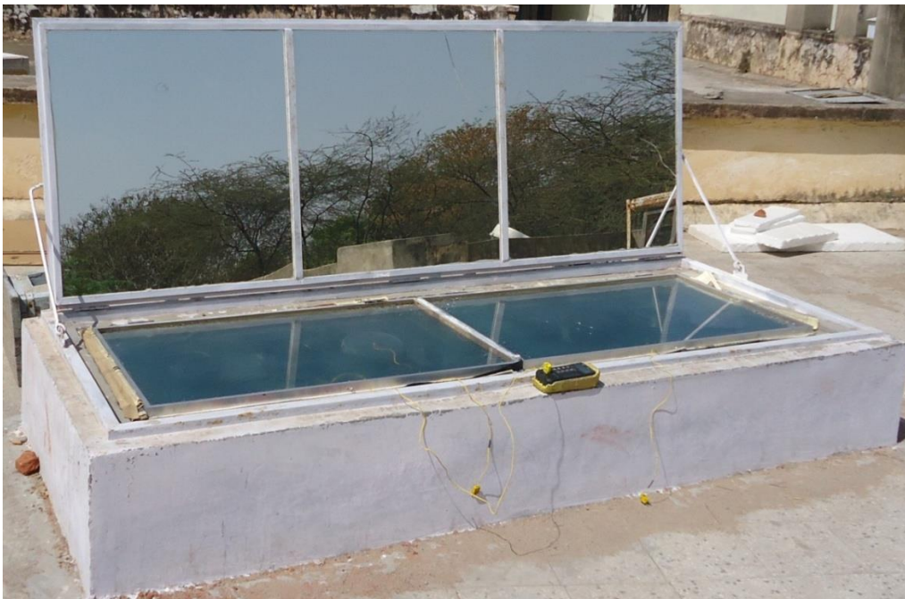
Photograph 1 On-field installation of developed community solar cooker.
